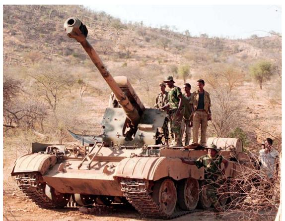
A self propelled gun made by assembling a 122mm MI 1963D30 gun- howitzer on the hull of a T54/55 10
